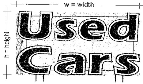
Calculating Area of a Sign where Copy Exceeds Sign Area = (height of copy) x (width of copy)
