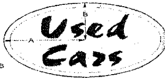
Calculating Area of an Elliptical Sign = \pi \times A \times B
